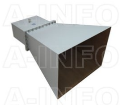
LB-2100-10-C-7/16F Standard Gain Horn Antenna 0.35-0.53GHz 10dB Gain 7/16(DIN) Female
